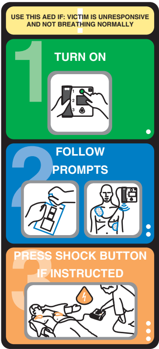
Fig. 5.1 AED power panel with prompts. (Courtesy Philips Medical Systems.)
