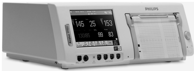
Fig. 3.3 Philips Avalon FM50 fetal monitor provides measurement of the fetal heart rate (FHR) including noninvasive triplet monitoring, FHR high/low audible and visual alarms, and fetal electrocardiogram (FECG). Maternal parameters include toco and intrauterine pressure, blood pressure, pulse rate, pulse oximetry, and ECG. It has cross-channel verification of maternal and fetal heart rate, displays FECG and maternal ECG on the color display touch screen, and has a LAN interface for compatibility with hospital IT networks. (Courtesy Philips Medizin Systemes, Böblingen, Germany.)
