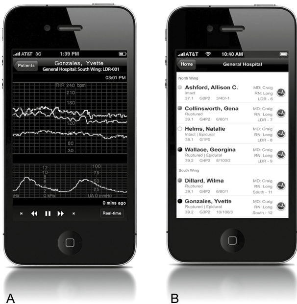
Fig. 3.20 Providers can access near real-time FHR tracings (A) and review patient data using their mobile phones (B). (Courtesy AirStrip Technologies, Inc., San Antonio, TX.)
