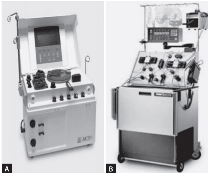
Figs. 10A and B: Plasmapheresis using the membrane and procedure separator.
