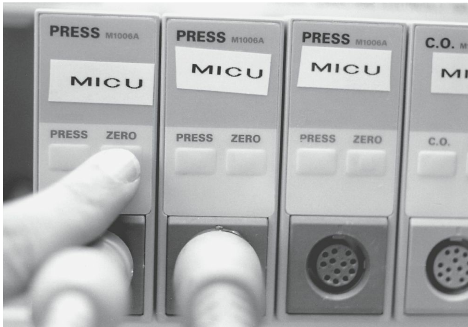
Figure 5-12. “Zeroing” a transducer.
